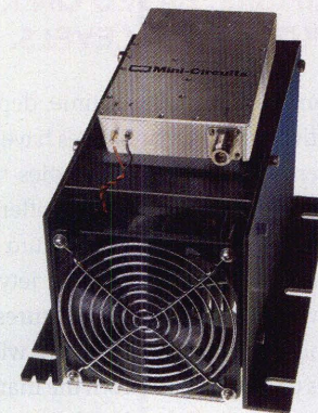
2. The large heat sink is required to help dissipate heat from the power amplifier's active devices. [Photo courtesy of Mini-Circuits ( www.minicircuits.com ).]
